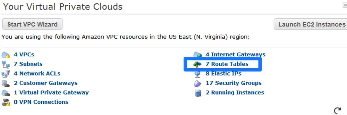
2. The available routing tables are displayed. In the screenshot below, the main routing table for the 70.0.0.0 VPC has no associated subnets. We want to ensure that both the public and private subnets are associated to the main routing table.
